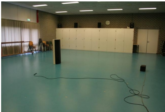
Figure 1. Ground Plane Measurement Method setup with speaker, microphone, and Device Under Test ( DUT)
